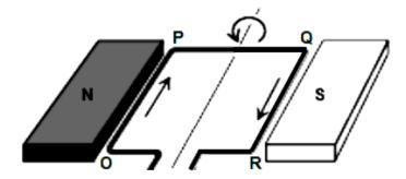
Which TWO segments of the loop will experience an electromagnetic force when the loop is in the position above?
