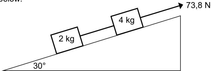
The magnitude of the kinetic frictional force on the 4 kg block is 20 N. The coefficient of kinetic friction applicable to the 2 kg block is 0,589.
