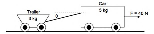
2.1.6 Draw a free-body diagram, with labels, of all the forces acting on the CAR. (5)
