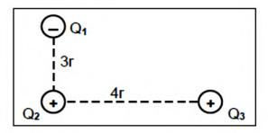
The magnitude of the charge on  $Q_1$  is nine times that of  $Q_2$  ( $Q_1 = 9Q_2$ ). The magnitude of the charge on  $Q_3$  is sixteen times that of  $Q_2$  ( $Q_3 = 16Q_2$ ). The distances between  $Q_1$  and  $Q_2$  and between  $Q_3$  and  $Q_2$  are 3r and 4r respectively.
