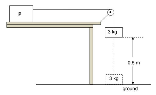
Initially the system of masses is held stationary with the 3 kg block, 0,5 m above the ground. When the system is released the 3 kg block moves vertically downwards and strikes the ground after 3 s. Ignore the effects of air resistance.
