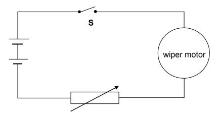
When switch **S** is closed, the potential difference across the variable resistor is 2,8 V and the current passing through it is 0,7 A.
