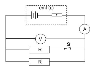
Switch **S** is now closed. How do the readings on the ammeter and voltmeter change?
