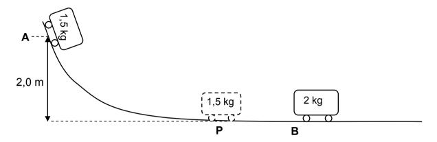
4.1 Use the principle of conservation of mechanical energy to calculate the speed of the 1,5 kg trolley at point **P**.
