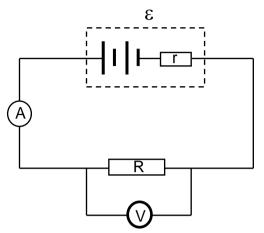
A second resistor with the **same resistance** as **R** is connected in parallel with **R**. How will the voltmeter and ammeter readings change when the second resistor is added to the circuit?
