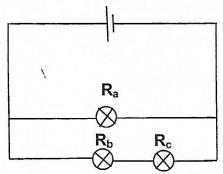
Which ONE of the potential difference combinations across bulbs  $R_a$ ,  $R_b$  and  $R_c$  respectively will be CORRECT?
