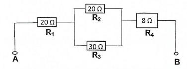
8.1 Calculate the total resistance between **A** and **B**. (3)
