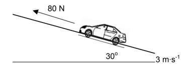
Use energy principles to calculate the speed of the car after it has travelled 5 m up the inclined plane.
