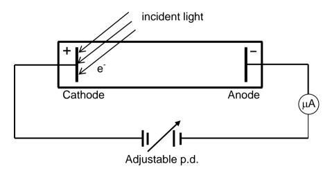
It was found that light of 500 nm releases electrons with zero kinetic energy. The microammeter gives a zero reading.
