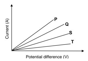
The resistor with the second largest resistance is:
