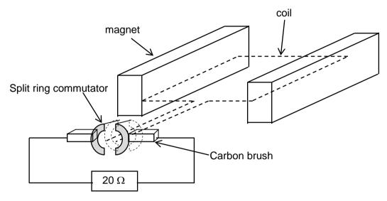
9.1 The coil rotates within the magnetic field.
