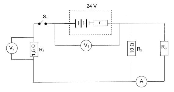
The resistance of  $R_1$  is 1,5  $\Omega$ , the resistance of  $R_2$  is 10  $\Omega$ , while the resistance of  $R_3$  is unknown.
