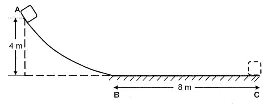
An object of mass 10 kg is released from point **A** which is 4 m above the ground. It slides down the track and comes to rest at point **C**.
