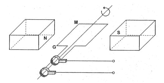
10.1 Determine the direction of the current in segment GM when the coil is in the position shown above. Only write down G to M OR M to G. (1)
