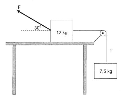
The maximum co-efficient of static friction( $\mu_s$ ), between the 12 kg block and the surface of the table is 0,45. Ignore the effects of air friction.
