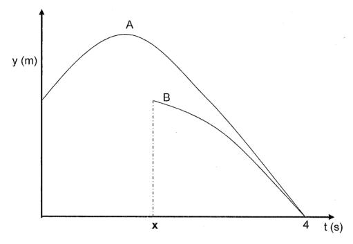
Stone A is thrown vertically upwards at 19 m.s<sup>-1</sup> and strikes the ground after 4 seconds. Stone B is dropped after **x** seconds and strikes the ground at the same time that stone A strikes the ground.
