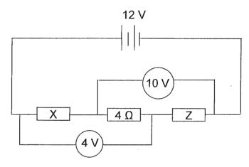
The battery has no internal resistance and the resistance of the conducting wires can be ignored.
