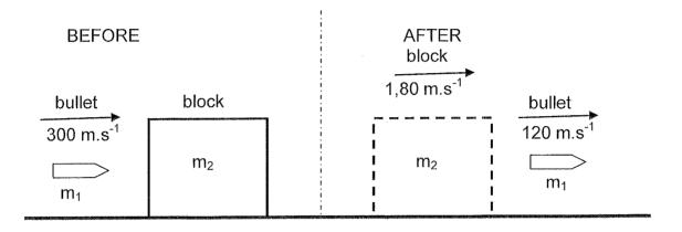
It is observed that the kinetic energy of the bullet – block system decreases by 752,76 J.
