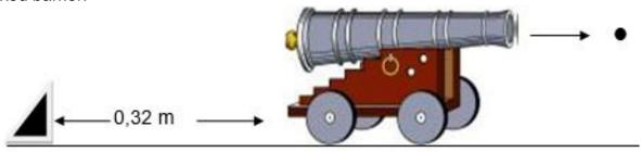
At the instant the steel marble leaves the canon, the canon starts moving backwards (recoils) at a **constant velocity**.
