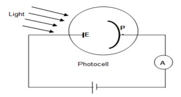
When the photocell is in the dark the ammeter reads zero. But when monochromatic red light with a frequency of 4.65 x 10<sup>14</sup> Hz from a 50 W bulb is shone on the photocell, a small current is registered on the ammeter.
