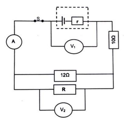
(3)Calculate the resistance of resistor R. 8.1 Calculate the reading on the ammeter. (5)8.2 Explain, in words, what is meant by the term internal resistance. (2)8.3 Calculate the potential difference across the 10  $\Omega$  resistor. (3)8.4 When switch S is opened, voltmeter V1 reads 45,9 V. Hence, 8.5 calculate the internal resistance of the battery. (5) Does the external resistance in the circuit INCREASE, DECREASE 8.6 or REMAIN THE SAME when the resistor R is removed? (1) [19]
