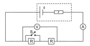
Which ONE of the following combinations CORRECTLY represents the change in the readings on the **ammeter** and the **voltmeter** when switch **S** is closed?
