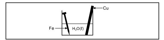
After a while it was observed that the iron nail was coated with rust. The copper rod showed no visible signs of corrosion.
