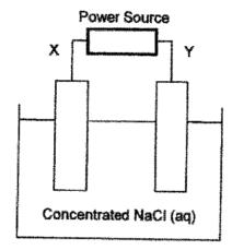
Chlorine gas is released at electrode Y.
