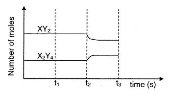
The value of Kc at BOTH TIMES t<sub>1</sub> and t<sub>3</sub> is 0,25.
