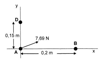
The net electrostatic force experienced by sphere **A** is 7,69 **N** in the direction as shown in the diagram above.
