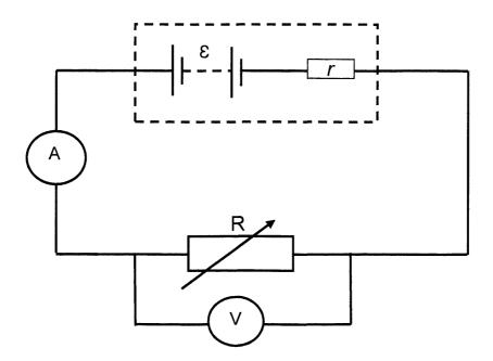
The resistance of the variable resistor R is INCREASED now.
