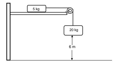
When the stationary 5 kg mass is released, the two masses begin to move. The coefficient of kinetic friction,  $\mu_k$ , between the 5 kg mass and the horizontal surface is 0,4. Ignore the effects of air friction.
