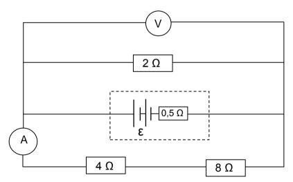
The reading on the ammeter is 0,2 A.
