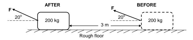
The coefficient of kinetic friction,  $\mu_k$ , between the floor surface and the block is 0.2.
