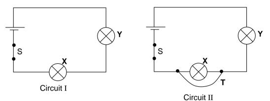
A wire  ${\bf T},$  of negligible resistance, is now connected across  ${\bf X}$  as shown in Circuit II.
